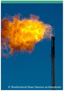
Flaring is the intentional burning of natural gas that often cannot be transported fast enough. In 2018, flaring in the U.S. alone was responsible for 32.8 million metric tons of carbon dioxide emissions.
